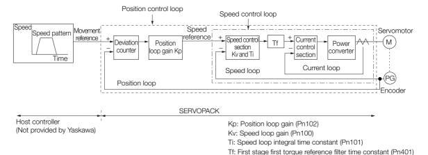
In order to manually tune the servo gains, you must understand the configuration and characteristic of the SERVOPACK and adjust the servo gains individually. In most cases, if you greatly change any one parameter, you must adjust the other parameters again. To check the response characteristic, you must prepare a measuring instrument to monitor the output waveforms from the analog monitor.
