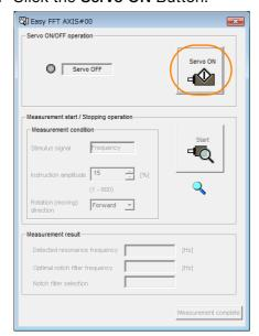
The motor shaft will rotate and measurements will start.
