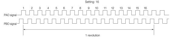
7.5.2 Setting for the Encoder Divided Pulse Output
