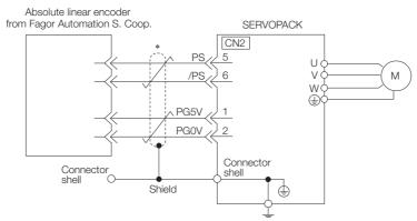
4.4.3 Wiring the SERVOPACK to the Encoder
