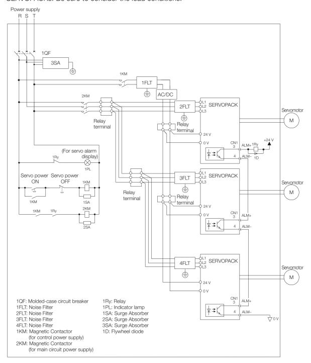
To comply with UL/cUL standards, you must install a branch circuit protective device at the power supply input section to each SERVOPACK. Refer to the following document for details.
