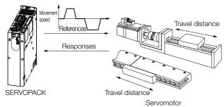
Note: Execute moment of inertia estimation after jogging to a position that ensures a suitable range of motion.
