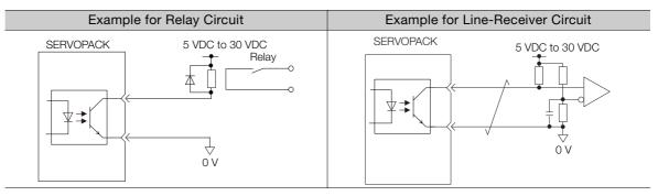
Note: The maximum allowable voltage and current range for photocoupler output circuits are as follows:
