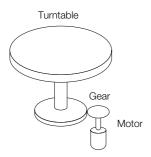
Because the turntable moves in only one direction, the upper limit to the number of rotations that can be counted by an absolute encoder will eventually be exceeded.
