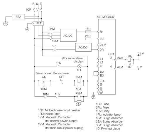
• Wiring Example for DC Power Supply Input: SGD7S-210D, -260D, -280D, and -370D
