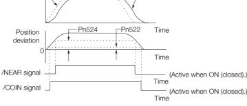
Note: Normally, set Pn524 to a value that is larger than the setting of Pn522 (Positioning Completed Width).
