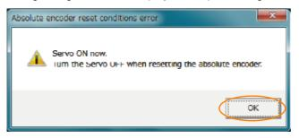
Click the **OK** Button. The Main Window will return. Turn OFF the servo and repeat the procedure from step 1.
