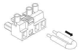
3. Remove the sheath from the wire to connect.
