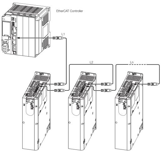
Note: The length of the cable between stations (L1, L2, ... Ln) must be 50 m or less.
