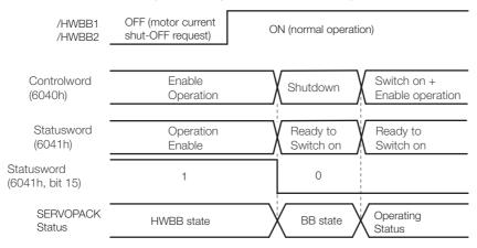
Note: If the SERVOPACK is placed in the BB state while the main circuit power supply is OFF, the HWBB state will be maintained until the Shutdown command is received.
