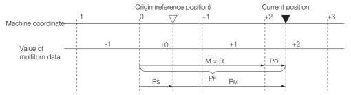
The current position  $P_M$  in the machine coordinate system is calculated as follows:
