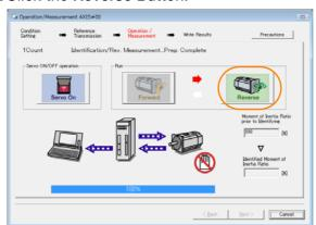
The shaft will rotate in the reverse direction and the measurement will start. After the measurement and data transfer have been completed, the **Forward** Button will be displayed in color.
