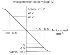
Note: The effective linearity range is  $\pm 8$  V. The resolution is 16 bits.
