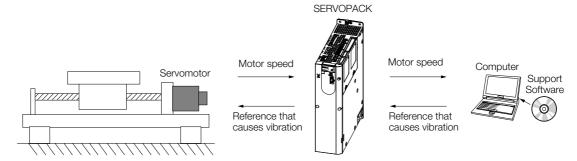
The motor is used to cause machine vibration and then the speed frequency characteristics for the motor torque are measured. The measured frequency characteristics can be used to determine the machine resonance.
