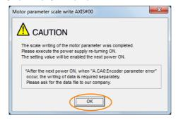
12. Turn the power supply to the SERVOPACK OFF and ON again.
