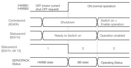
If the /HWBB1 and /HWBB2 signals are OFF and the Servo ON command (Enable Operation command) is received, the HWBB state will be maintained even after the /HWBB1 and /HWBB2 signals are turned ON.
