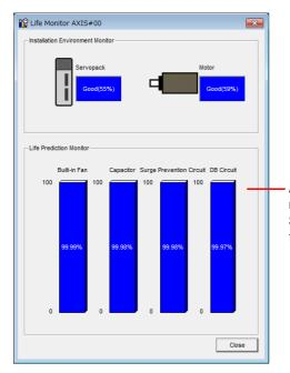
A value of 100% indicates that the SERVOPACK has not yet been used. The percentage decreases as the SERVOPACK is used and reaches 0% when it is time to replace the SERVOPACK.
