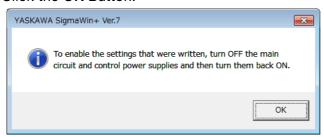
8. To enable changes to the settings, turn the power supply to the SERVOPACK OFF and ON again.
