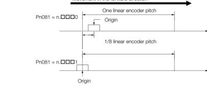
Observe the following precaution if you set Pn081 to n. \$\square\$ (Output phase-C pulses only in the forward direction).
