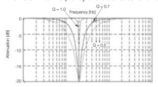
Note: The above notch filter frequency characteristics are based on calculated values and may be different from actual characteristics.
