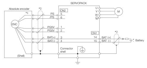
\*1. The absolute encoder pin numbers for wiring the connector depend on the Servomotor that you use.
