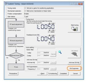
3. Click the Import Button or click ▲ and ▼ Button to manually adjust the set frequency. When you click the Import Button, the residual vibration frequency in the motor is read as the set frequency. (The frequency can be read only when the residual vibration frequency is between 1.0 and 100.0.)
