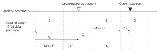
The current position  $P_{M}$  in the machine coordinate system is calculated as follows:
