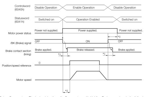
\*1. Rotary Servomotors: The brake delay times for Servomotors with Holding Brakes are given in the following table. The operation delay times in the following table are examples for when the power supply is switched on the DC side. You must evaluate the actual brake delay times on the actual equipment before using the application.
