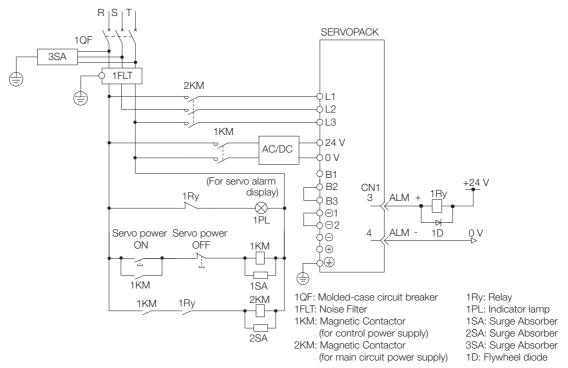
Wiring Example for Three-Phase, 400-VAC Power Supply Input: SGD7S-210D, -260D, -280D, and -370D
