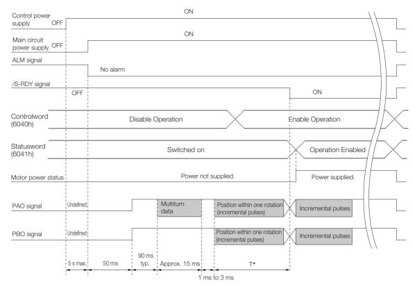
\* The pulse output time T for the position of the absolute encoder within one rotation depends on the setting of Pn212 (Number of Encoder Output Pulses). Refer to the following table.
