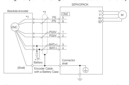
\*1. The absolute encoder pin numbers for wiring the connector depend on the Servomotor that you use.
