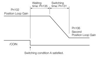
Information You can use gain switching for either PI control or I-P control (Pn10B =  $n.\Box\Box\Box\Box$  or  $\Box\Box\Box\Box\Box$ ).
