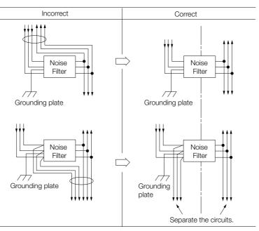
• Separate the Noise Filter ground wire from the output lines. Do not place the Noise Filter ground wire, output lines, and other signal lines in the same duct or bundle them together.
