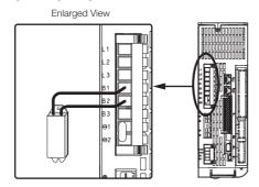
Set Pn600 (Regenerative Resistor Capacity) and Pn603 (Regenerative Resistor Resistance).
